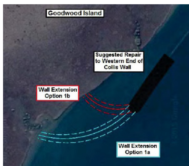
Figure 7: Extension of wall to protect erosion at Goodwood Island
